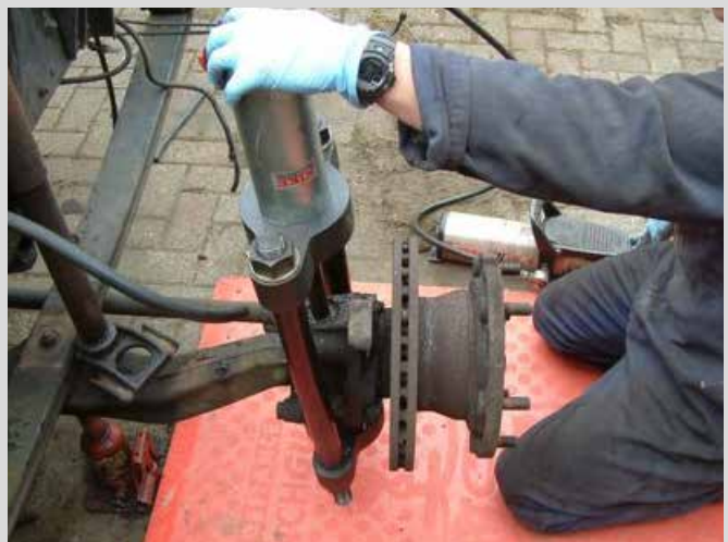
Replacing a seized king pin can be a time consuming process. Using the KPP20 means keeping trouble and labour time for this kind of job to a minimum.
