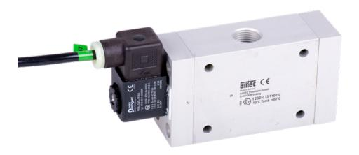
Electrically operated valves conform to equipment category 2 can be used in Zone 1 respectively in Zone 21. For the use in hazardous areas the category group of the used coil has to be taken into account. The specification of the whole equipment corresponds always to the lowest category of the single components.
