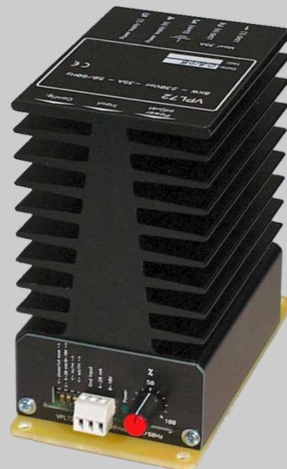
**Power controller with analog command. The output modulation can be phase angle variation or burst fired (zero-cross), allows extremely fine and fast modulation of resistive loads even with low thermal inertia as infrared.**
