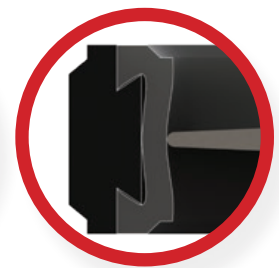
Poor: Booted Seat bulging around disc contact points
